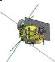
Downlinks for A2 would be 435.400 MHz and 436.400 MHz using 10K0F1DCN or 10K0F1DEN (10-kHz wide FM single-channel data) 250 bps GMSK with concatenated codes or JT65B.
